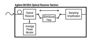
The integrated optical channel can be used as a fully calibrated SONET/SDH/Gigabit Ethernet or Fibre Channel reference receiver or a wide-bandwidth receiver.
